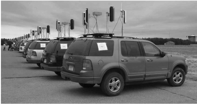
Fig. 7. Row of demo 1 vehicles. Mounted on top of each vehicle are four directional antennas, an omni antenna, and a mast holding the GPS device away from the vehicle.
