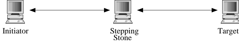
Figure 6: Three hosts used to test stepping stone detection algorithms. The initiator establishes an interactive remote login connection to the stepping stone, and from the stepping stone another interactive remote connection is established to the target.
